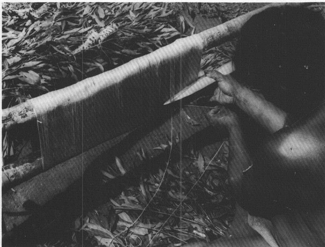
FIG. 64. First insertion of the weft which is started some distance in from the right selvage, then carried to that selvage before being carried to the left. Note that only about eight warp are lifted by the pickup-beater tool.
